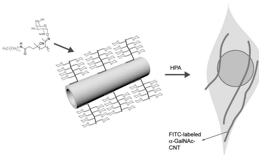
**Fig. 2** A CNT coated with biomimetic carbohydrate polymers to mimic cell surface mucin glycoproteins. The CNTs can bind to mammalian cells specifically with the aid of a hexavalent lectin, HPA.
